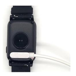
Back of Unit Connect Magnetic Cable for Charging
